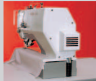
Servo sewing drive integrated in housing
