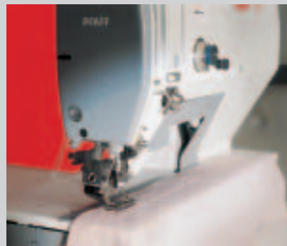
Off-set arm for easy placing/handling of workpiece
