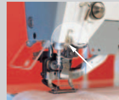
Thread monitor with optical sensor
